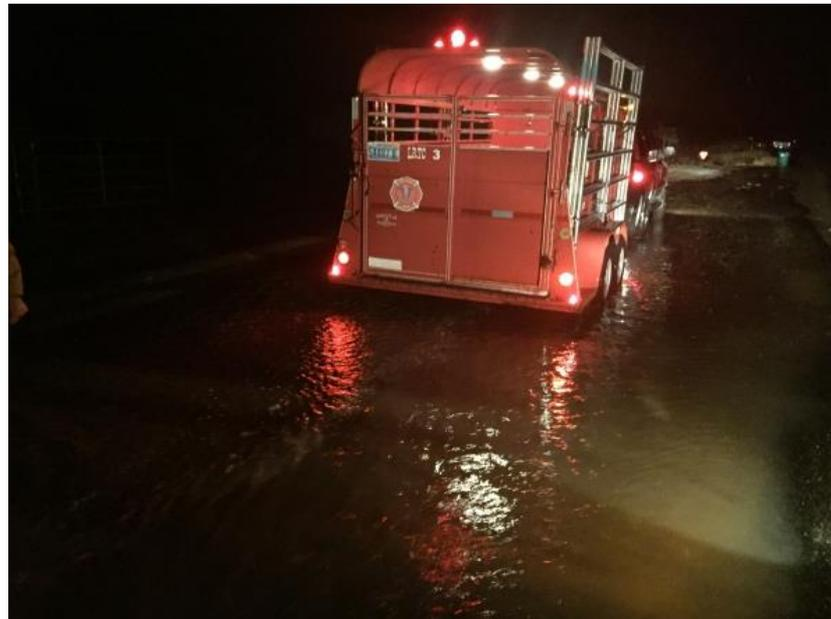
Auxiliary amber stop and turn signal lamps are recommended on trailers where factory tail / stop / signal lamps are mounted low.
